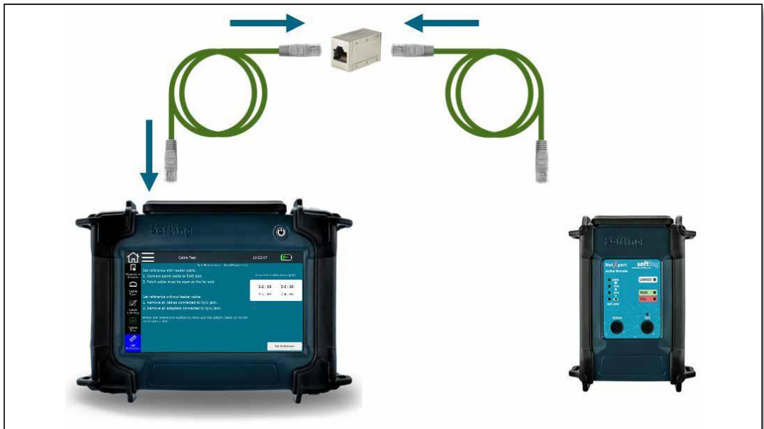
Figure 39 - Test setup for setting the reference - Cu
